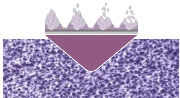
The Ceramic grains of this line provide long-lasting sharp edges, offering better finishing results on the treated surfaces. The 740 Ceramic products are perfect for sanding any type of material, such as scratch resistant varnishes and e-coats, primers and composites, eliminating the need for specialty products.
