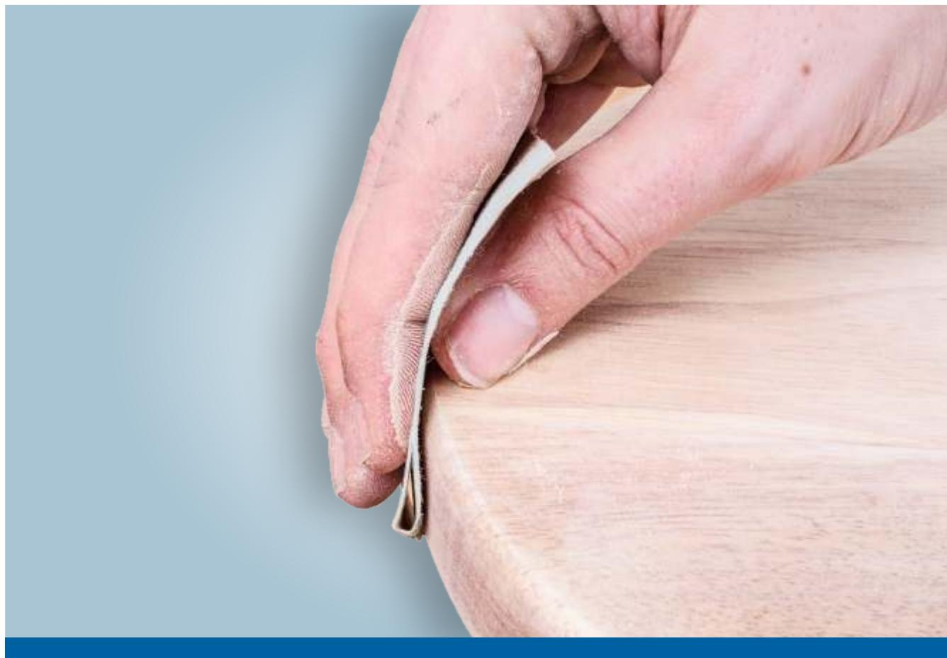
The 140 SIC Finishing sheets are suitable for wood sanding and veneer finishing. The Silicon carbide grains feature fine stock removal and a uniform scratch pattern, whilst the open coat structure and the stearate top coat prolong their lifespan, preventing them from clogging.
